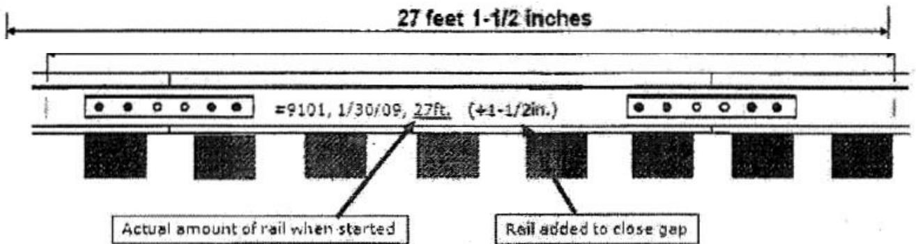
When returning to correct the lowered rail neutral temperature or making the welds for a rail plug that was calculated to be within the rail installation safe range, the information on the rail provides the information needed to close out the location correctly. The original reference mark length, gap distance, and rail temperature at the time of separation, are needed to make these adjustments.
