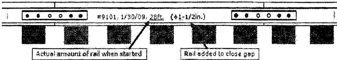
In cases of pull-a-parts and service failures where the rail has gapped open, the distance of reference marks on the web of the rail must not include the gap in the rail. The reference marks should always indicate the original distance, (amount of rail) between the marks before the break or pull-apart occurred. In this example the gap is 1 ½" wide and the break is crooked.
