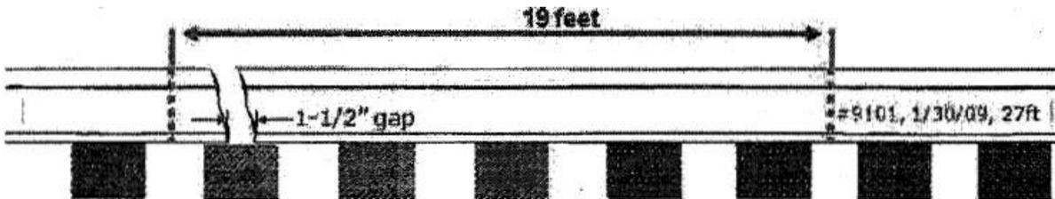
Once the temporary repair (filled the gap) is completed, measure the distance between the reference marks and record the amount of change on the web of the rail.
