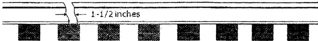
Decide where to make saw cuts (preferably away from the break). Measure back from those cuts at least 3', and make the reference marks. Measure the reference mark distance, and then subtract the amount of gap to get the original reference mark distance.
